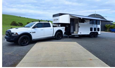
Composite fibreglass foam core walls, roof & barn doors for very high strength. These floats are lightweight, FULLY INSULATED with smooth clean finishing's internal and external.
